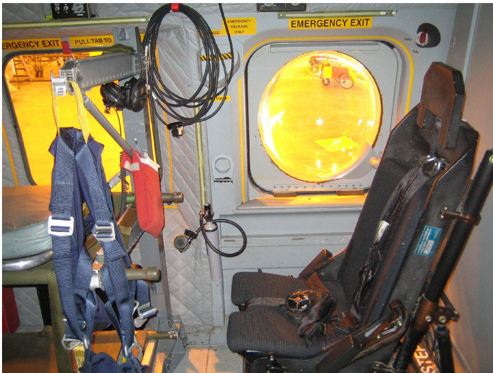
Photograph 11: Anchor Strap attachment point to restraint harness.
