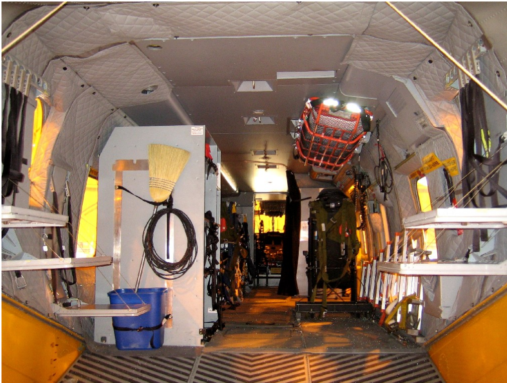
Photograph 6: Standard SAR configuration layout, looking at the left side of the cabin.
