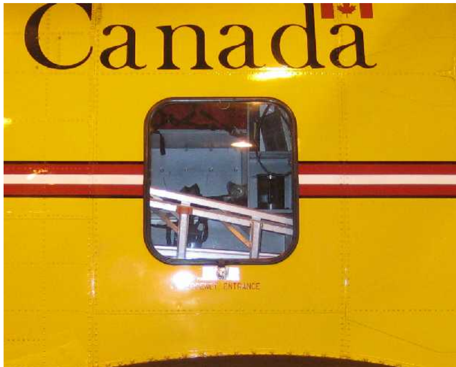
Photograph 8 : Secondary exit with external view with the ladder positioned as it was found, blocking the exit in CH149914
