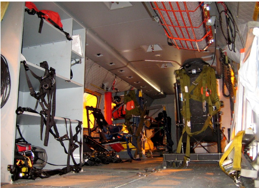
Photograph 6: Standard SAR configuration layout, looking at the left side of the cabin.
