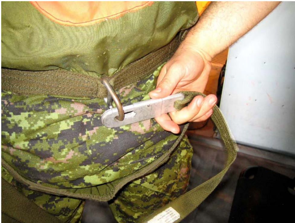
Photograph 11: Anchor Strap attachment point to restraint harness.
